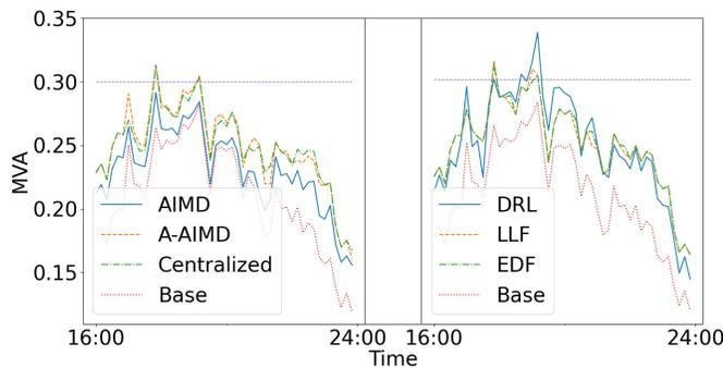
Fig. 4: Loading of a distribution transformer under centralized, A-AIMD and AIMD algorithms (right figure), and DRL, LLF and EDF strategies (left figure). The dashed horizontal line is the rated capacity and the red curve is the base load.
