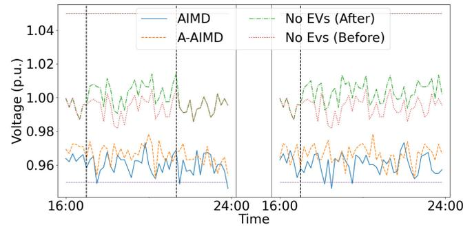
Fig. 8: Voltage profile of Node 18 under A-AIMD and AIMD algorithms. In the left plot the substation voltage increases between 5:00pm and 9:00pm (marked by dashed vertical lines). In the right plot the configuration is changed (reconfiguration A) at 5:00pm (marked by the dashed vertical line).
