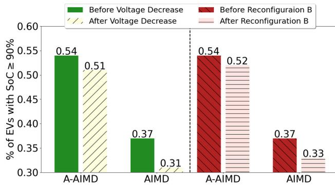
Fig. 11: Performances of A-AIMD and AIMD before and after voltage decrease (left panel) and after reconfiguration B (right panel). Note that the y-axis is truncated.
