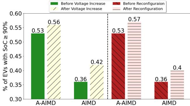
Fig. 10: Performances of A-AIMD and AIMD before and after voltage increase (left panel) and after reconfiguration A (right panel). Note that the y-axis is truncated.
