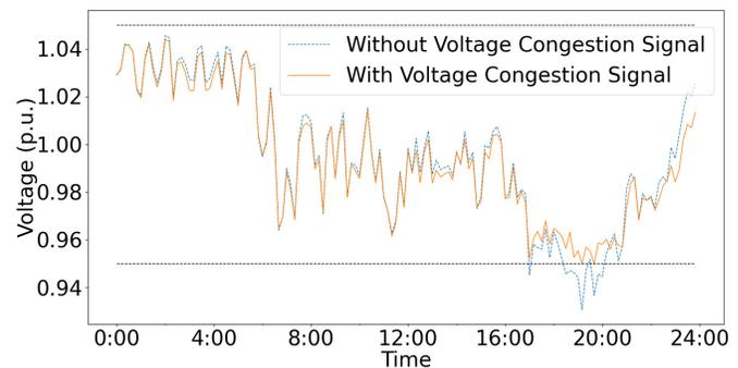
Fig. 5: The voltage of one of the primary nodes of the distribution network using A-AIMD with and without considering voltage congestion signals. The horizontal lines indicate  $\pm 5\%$  of the nominal voltage.
