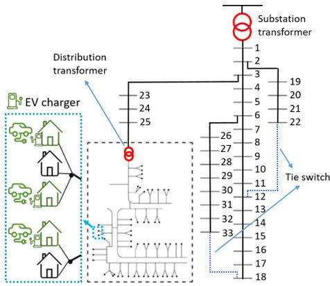
Fig. 1: The primary distribution network (Nodes 1-33) and secondary feeders (one of them is shown inside the dashed rectangle) supplying residential loads and EV chargers.
