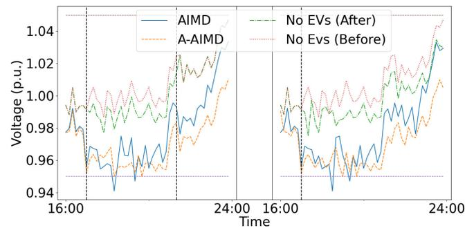
Fig. 9: Voltage profile of Node 33 under A-AIMD and AIMD algorithms. In the left plot the substation voltage decreases between 5:00pm and 9:00pm (marked by dashed vertical lines). In the right plot the configuration is changed (reconfiguration B) at 5:00pm (marked by the dashed vertical line).
