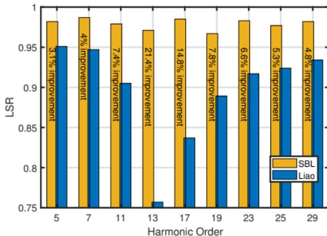
**Figure:** Comparing LSR of Lasso and SBL for different harmonic order under  $M_a$ . The LSR increased by **8.3%** on average.
