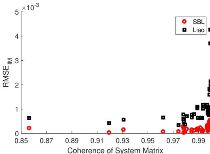
**Figure:** RMSE of the proposed state estimator versus Lasso with 9 harmonic meters when the system matrix has weak orthogonality.
