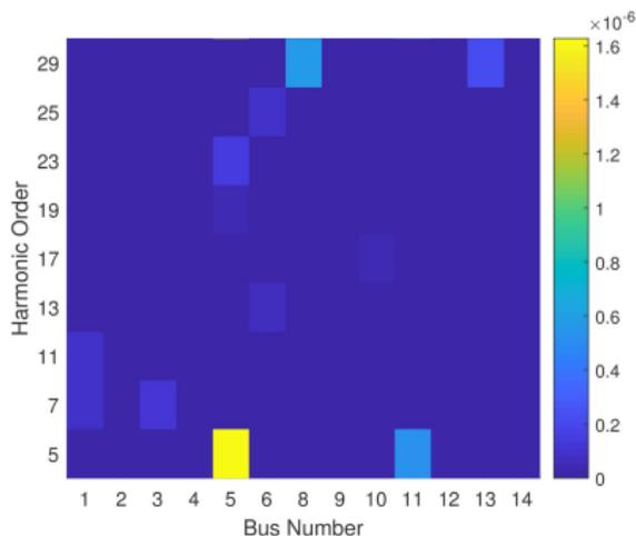
**Figure:** The identification error of injected current magnitudes for the meter configuration  $\mathbb{M}_a$  [2] in the noise-free scenario.
