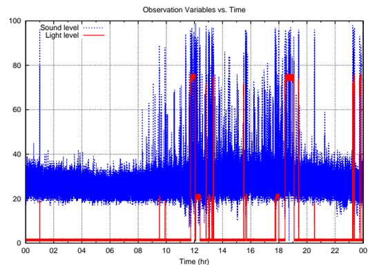
Figure 1: Sound and light measurement for a day
