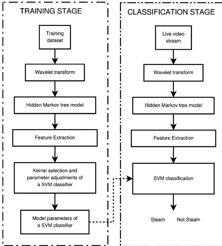
Fig. 2. Flowchart of the technique for the detection of steam in oil sand video images. In the training stage, the parameters of an SVM are determined by using a grid-search procedure.
