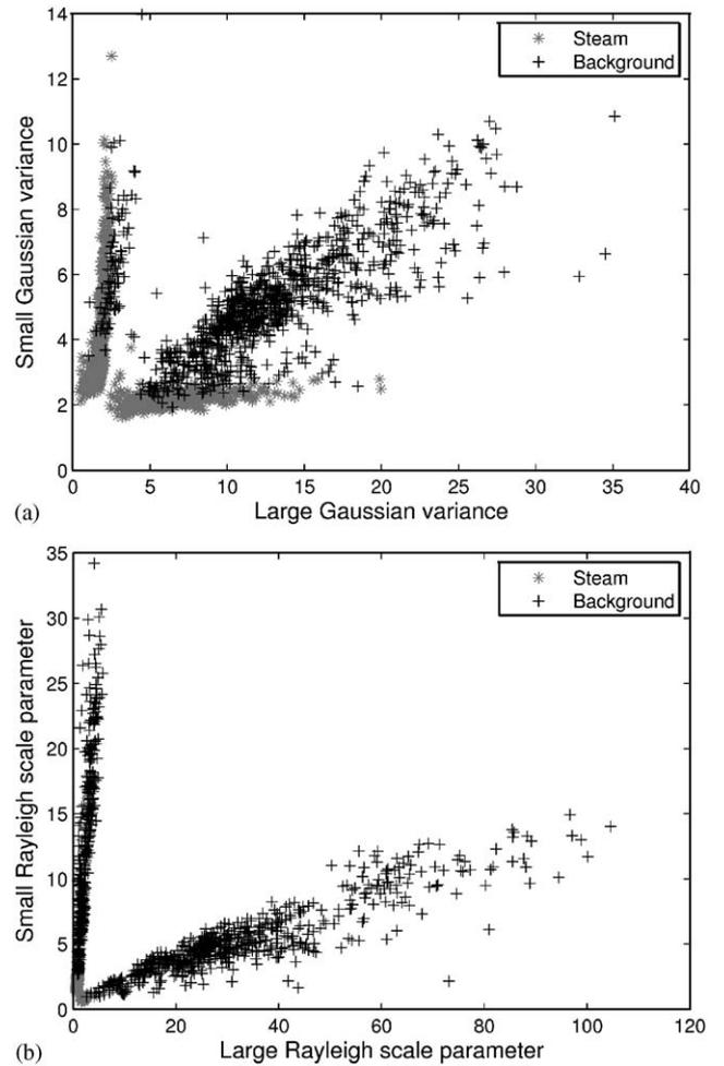
Fig. 4. Scatter plot of the Gaussian and Rayleigh parameters used in the current work as features on the detection of steam and background of the reject chute video images. (a) Large and small variances of the two-Gaussians fitting the marginal distribution of the DWT coefficients. (b) Large and small scale parameters fitting the marginal distribution of the DT-CWT coefficients.
