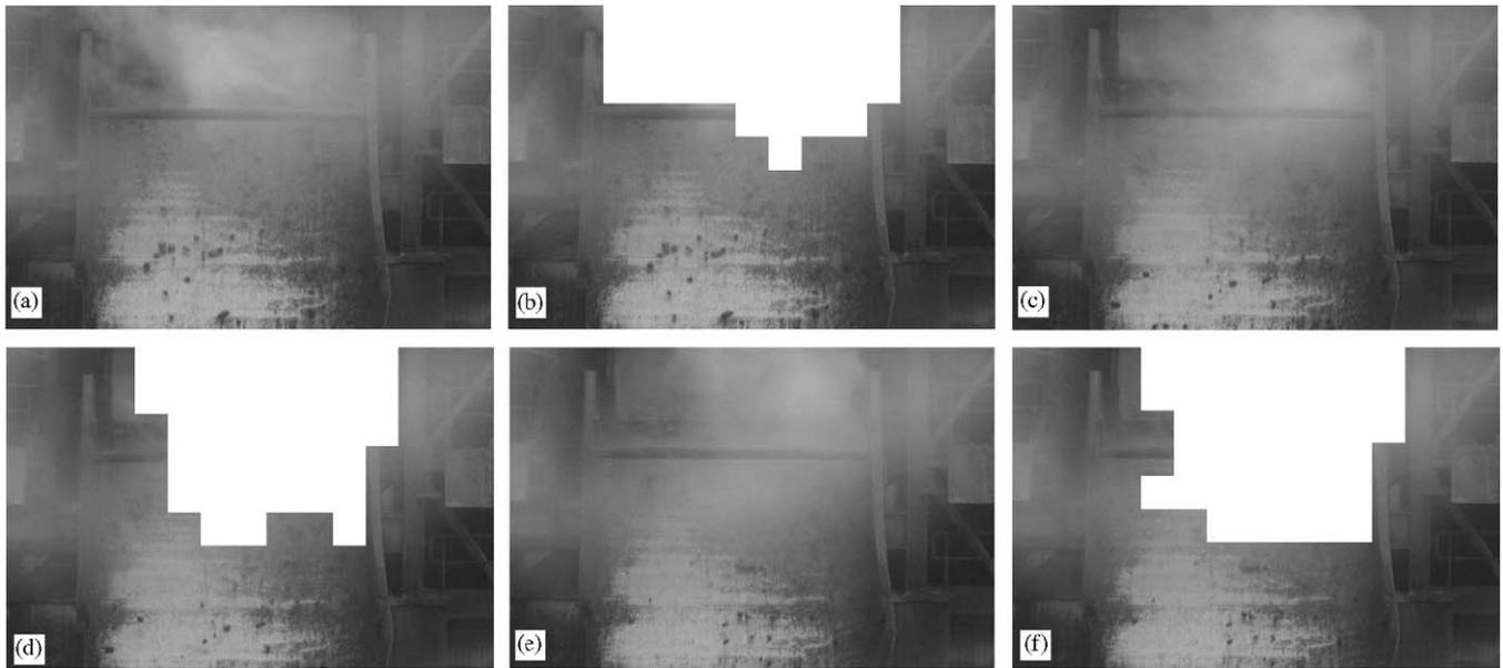
Fig. 7. Sequence of frames from a reject chute in a Syncrude mine—view 1. Left: original images. Right: results of the steam classification using the proposed algorithm.
