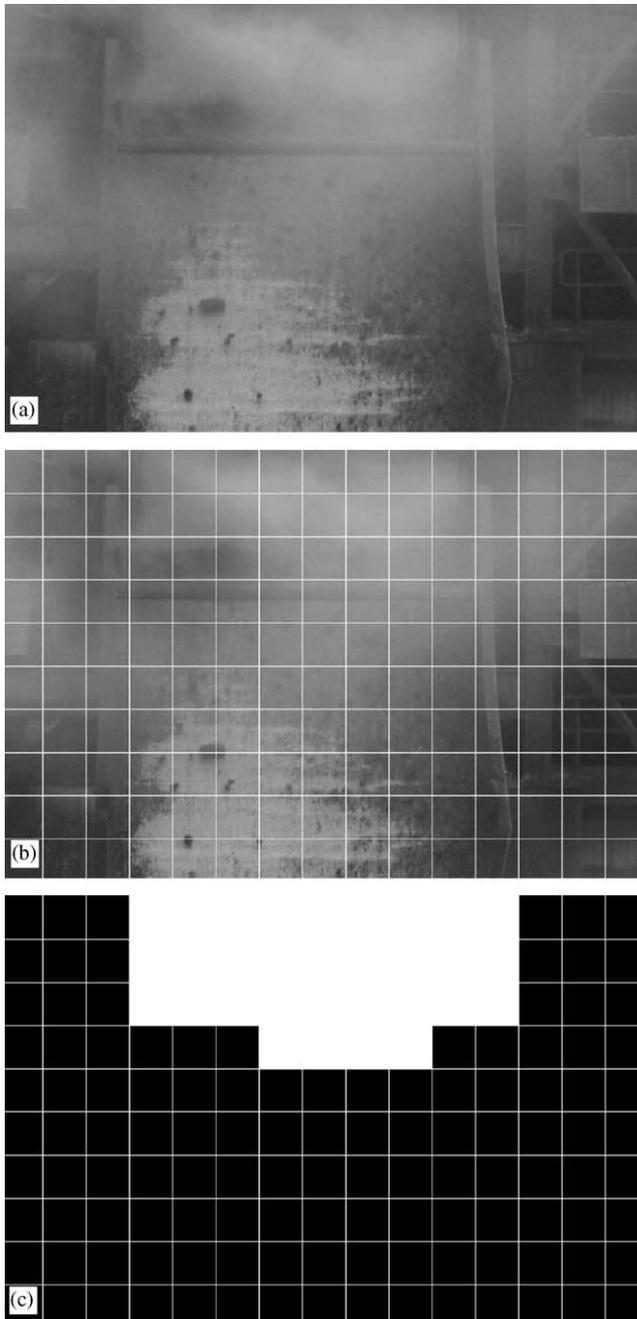
Fig. 6. Example of a frame image with steam used to assess the performance of the algorithm for detection of steam. (a) Original image. (b) Square-grid used to label the image overlaid on the original image. (c) Result of the visual classification.
