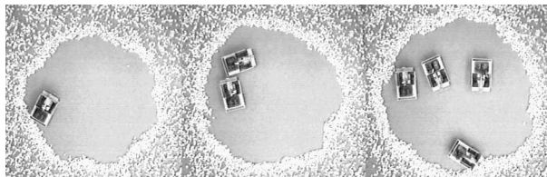
Figure 7: Nests constructed by one, two and four robots after two hours. The nest retained its initial circular shape and has uniform walls because the blind bulldozers enlarge the nest by distributing their pushes against the nest wall along its entire length.
