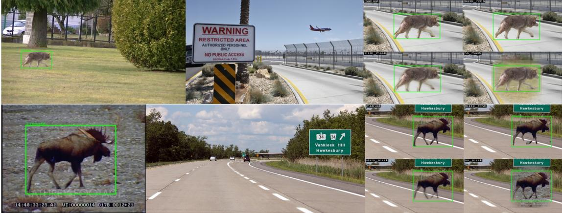
Figure 4.2: Synthetic data samples with corresponding source and target images for (top) coyote on airport and (bottom) moose on highway. Each row shows (left to right) animal source image, target background image and crops of synthetic images generated using (clockwise from top left) manual labeling, Mask RCNN, Gaussian blending (no mask) and SiamMask.
