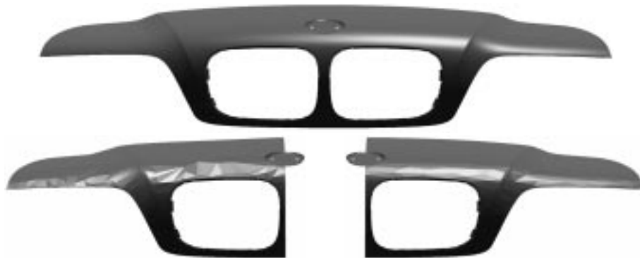
Figure 4.12. A dense mesh (top) is reduced with two different cost functions (bottom left: distance measure only; bottom right: distance measure and curvature dependent cost function).
