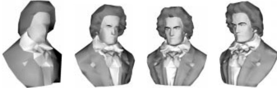
Figure 4.8. A coarse mesh with 256 triangles (left) is successively refined by adding vertices and triangles until the original mesh with 5030 triangles is reconstructed exactly (right).
