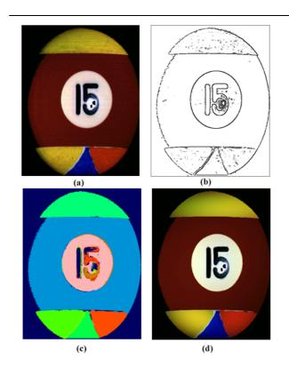
Figure 1. Segmentation of color range images of a billiard ball: (a) 3–D view of the color range image (b) detected range and color edges, (c) segmented image regions, (d) reconstructed color range image.
