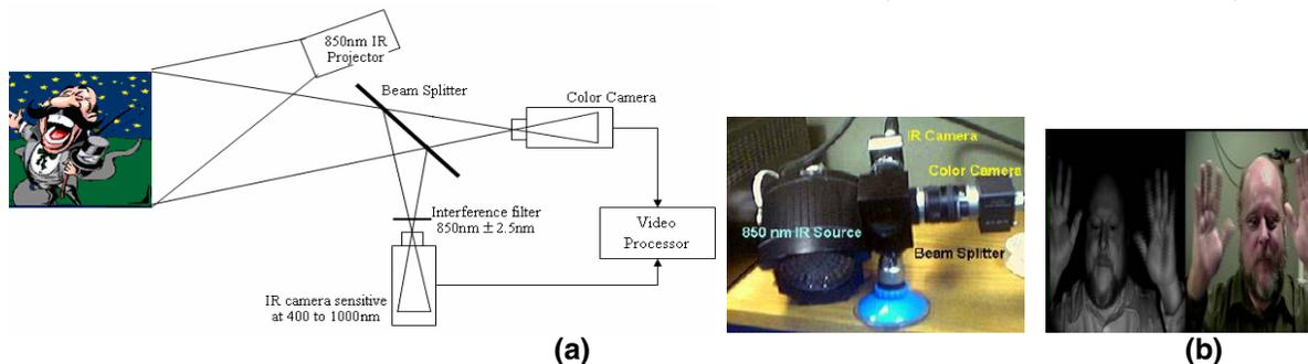
Figure 1: (a) Data acquisition unit (from [10]). (b) An example of a video frame.
