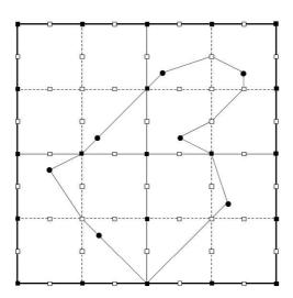
Figure 18.5: A portal-respecting tour(p-tour). Note that only black portals are used to enter or exit the level 1 squares, while the portals on the level 2 squares are added to enter or exit the level 2 squares.
