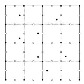
Figure 18.4: Portals added to the squares of the dissection with portal parameter m=2. The black squares are portals for both the level 1 and level 2 squares; the white squares are portals for the level 2 squares.
