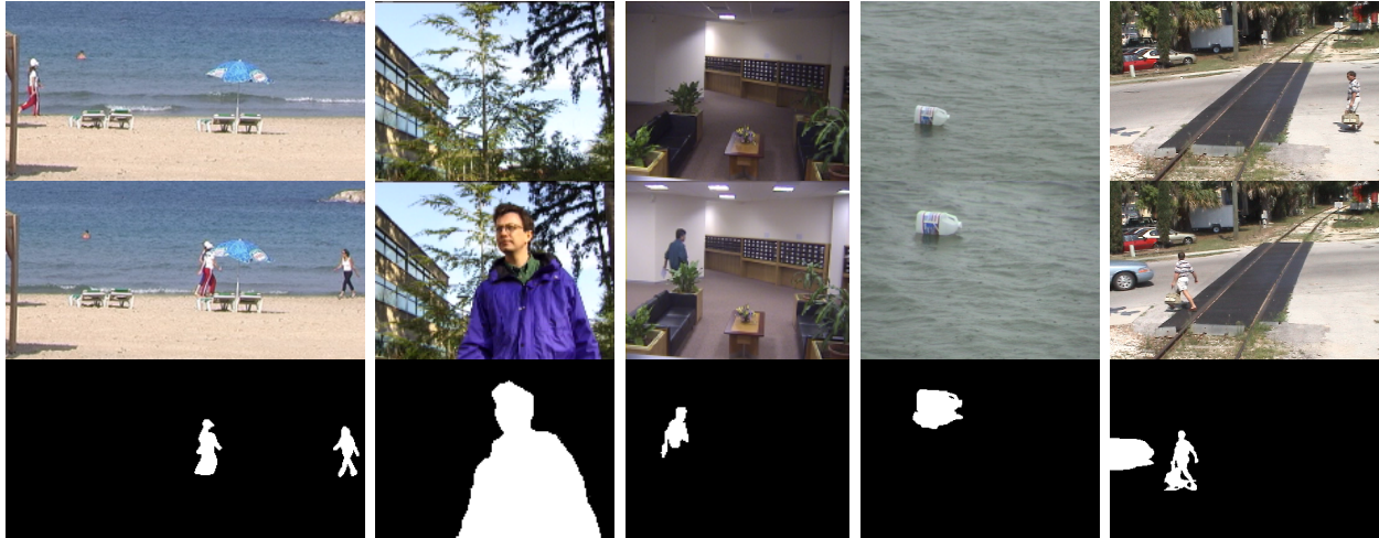
Fig. 8: Five datasets: (from left to right) Beach , Trees , Lights , Jug , and Railway . Top row: first frame in the sequence; Middle row: one key frame; Bottom row: hand-labeled foreground mask.
