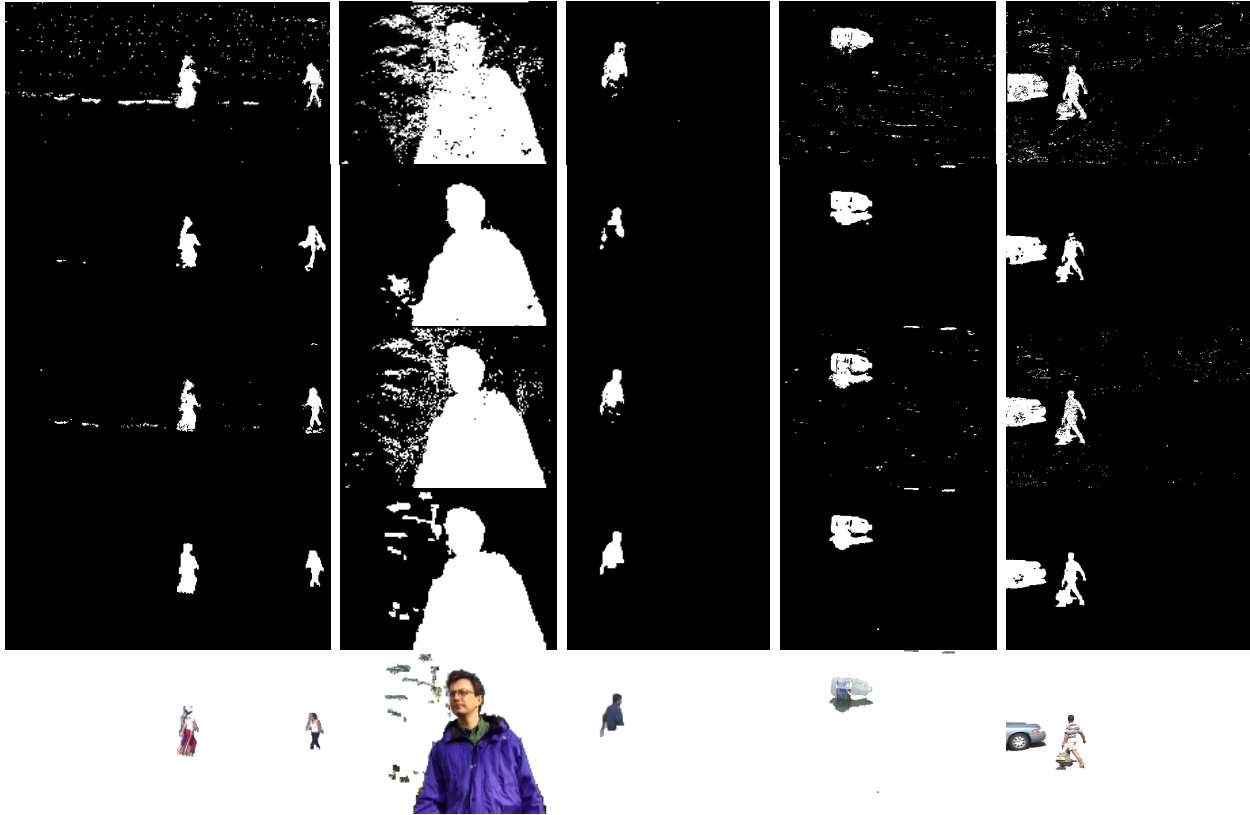
Fig. 9: First row: Results of MoG. Second row: Result of Sheikh et al. [22]. Third row: Results of SILK. Fourth row: Results of SILK-GC, and the results with foreground masks in Fifth row. Compared with SILK, SILK-GC effectively removes noises, and at the same time preserves the detailed shapes of foreground objects, e.g. the pedestrian in the Railway dataset.
