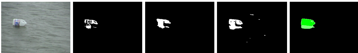
Fig. 11: Comparisons to other recent offline methods on the Jug dataset. From left to right: test frame, result from Figure 5 of [21], result from Figure 4 of [18], our result, and ground truth from Figure 4 of [18].
