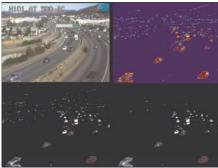
**Figure 5:** This figure presents, in scan-line order, the observed image, the confidence map, the result without false suppression and the result with false suppression, of the SILK algorithm on one road traffic sequence of frame 1552.
